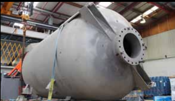
Ion Exchange vessel for NZ Refinery
