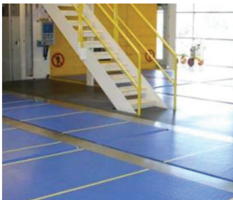
Photo above. Existing system, marking of belt edges will improve operator safety.
