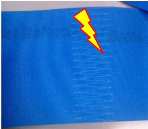
AS carbon warp ends interrupted by straight finger splice
